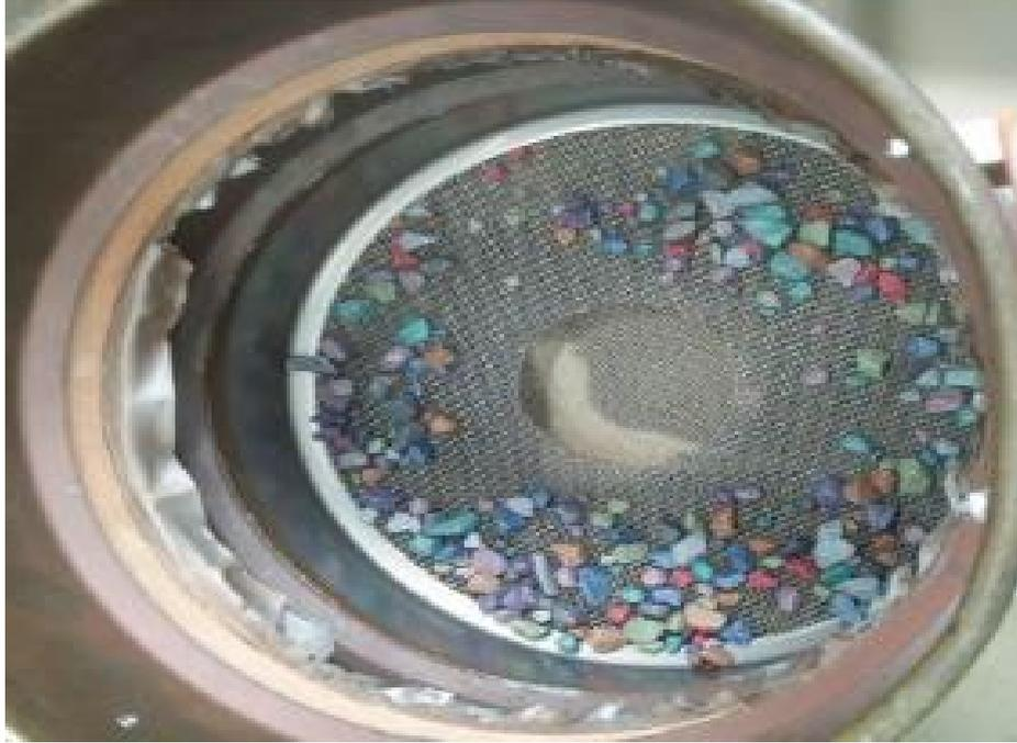
**Figure 3:** Photo of a mixture of the 2.0-8.0 mm tracer particles of nine different densities (distinguished by their colour) placed on the top screen mesh with 60 mm Sink-Hole. The second mesh visible beneath collects the underflow particles and helps suppress bubbling.
